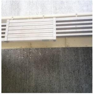
A longitudinal tining kit mounts to the adjustable transverse tine cart track located on the lower cord of the main frame. Standard tine rakes sections are clamped to a support pipe that can be hydraulically raised and lowered by the operator. Longitudinal tining and curing can be done concurrently. Because of the superior steering ability of the G&Z's TC1500, the longitudinal tining system delivers straight, uniformly spaced grooves.
